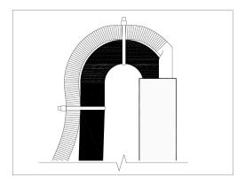
Secure the pump hose to the washer drain hose with 2 supplied cable ties as shown.
